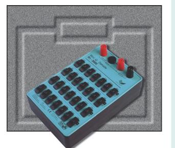
The R1-3000 compared to the R1-1000 offers a higher maximum power rating of 3 W. Additionally, the decade can be protected from an overload by using a quick-acting fine-wire fuse (a 400 mA fuse is supplied as standard accessory). By a non-fused resistance tap the internal resistance of the fuse can be by-passed. This ensures accuracy, particularly when low resistance values are concerned.
