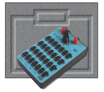
The RT1-1000 has the same technical features as the R1-1000. However, apart from the adjustment of resistance values it can also act as a voltage divider. A switchable tap allows the division of a total resistance of 156 kOhm into 156 kOhm / 0 kOhm, 100 kOhm / 56 kOhm, 150 kOhm / 6 kOhm, 156 kOhm / 0 kOhm. There are 6 switching positions in total for a real resistance division.
