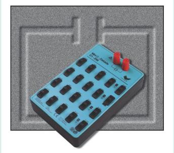
The C1-250 renders capacitance values in a range of 5 decades: 100 pF – 11,111  $\mu$ F. A staggering of the capacitors in 1-2-3-4 steps allows an airtight adjustment by means of sliding switches. The tapped value equals the sum of the adjusted capacitance values. The capacitor is automatically discharged when the corresponding slide is switched off. The supply is through 4 mm safety sockets.
