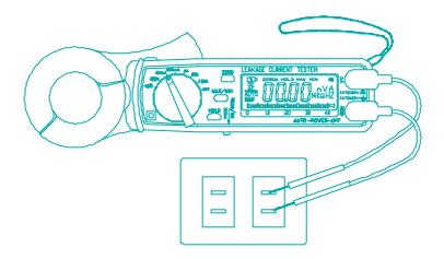
**WARNING:** Maximum input for DC V is 600, and for AC V is 600. Do not attempt to take any voltage measurement that exceeds the limits. Exceeding the limits could cause electrical shock and damage to the clamp meter.
