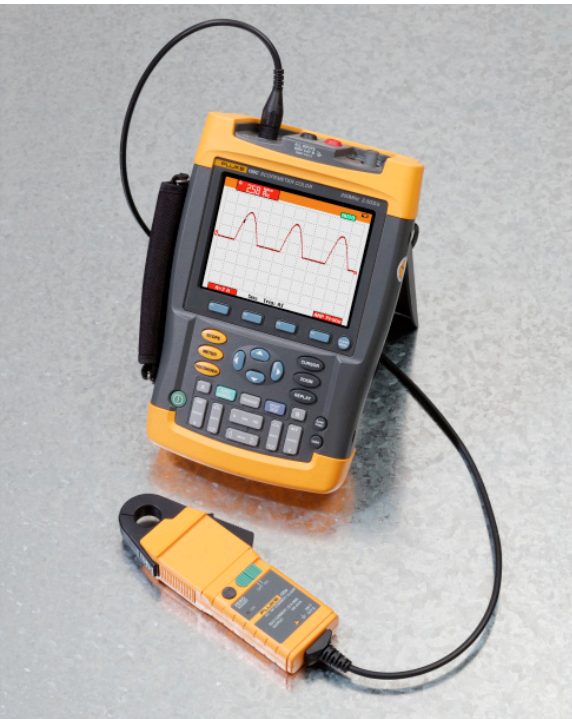
Fluke i30s connected to a Fluke 199C ScopeMeter.
