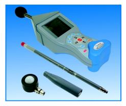
Additional measurement features are: a luminance measurement, a contrast, a globe temperature, a thermocouple (contact temperature), a PMV (predicted mean vote), a PPD (predicted percentage of dissatisfied), a WBGT (wet bulb globe temperature).
