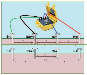
Wenner method: the distances between the 4 rods are identical: (d) ?W=2. ?.d.RS-SE
