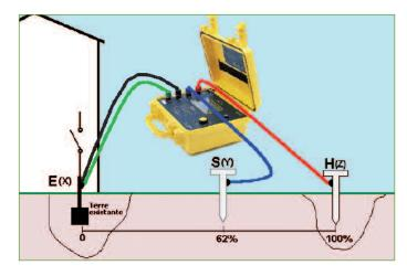
The 4P measurement method is more accurate and can be used to measure low earth resistances.
