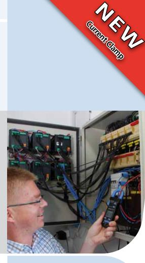
The MD 9225 is a versatile current clamp meter with perfect combination of size and built-in functions. It measures AC/DC current and voltage, capacitance, temperature, full range resistance and captures In-rush current. Display with large easy-to-read figures and one-handed operation make MD 9225 an extremely easy-to-use. This compact instrument combines a high level of functionality, small size and portability. All built-in features make MD 9225 a perfect tool for advanced applications.
