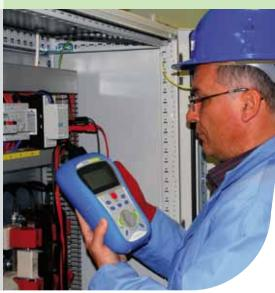
MI 3242 MicroOhm 2A is a portable low resistance ohmmeter used to measure low resistances of switches, relays, connectors, bus bars, power distribution cable joints, motor & generator winding, power transformers, power inductors, rail track joints, wire and cable resistance, welding joints for industrial application, etc., with test current up to 2A
