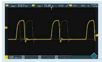
The high-speed acquisition system of the R&S<sup>®</sup>Scope Rider captures up to 50 000 waveforms/s and uncovers rare and unexpected signal anomalies.
