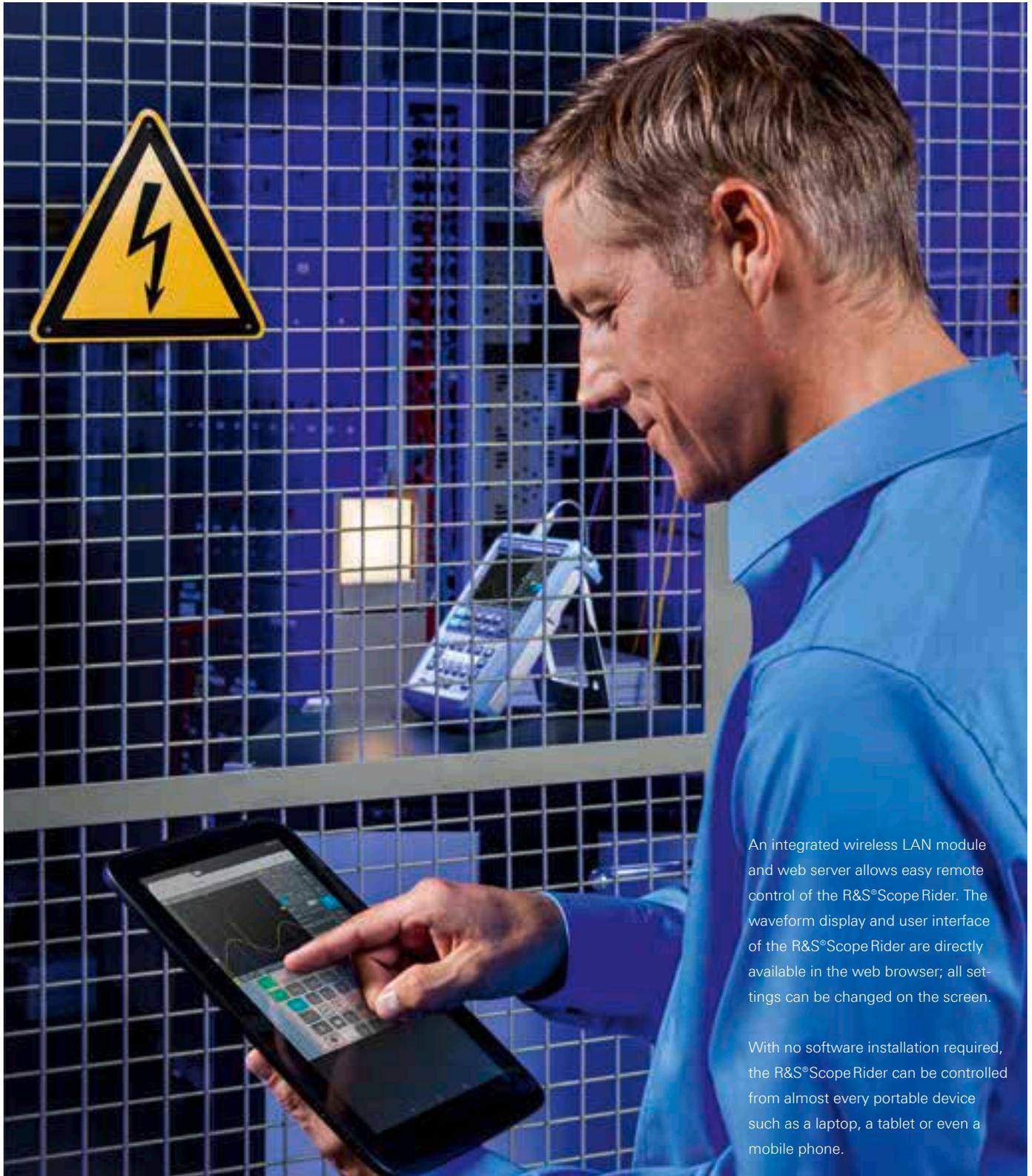
An integrated wireless LAN module and web server allows easy remote control of the R&S®Scope Rider. The waveform display and user interface of the R&S®Scope Rider are directly available in the web browser; all settings can be changed on the screen.
