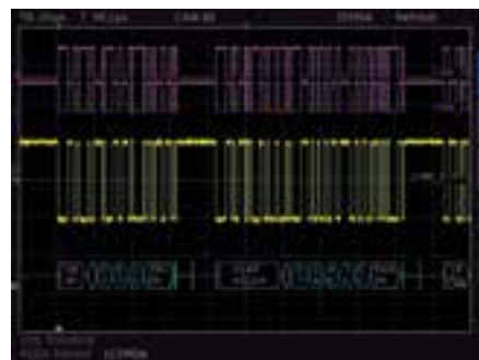
HEX decoded CAN bus signal.
