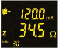
Screen 1: Impedance and leakage current
