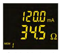
Standard mode: Impedance and leakage current
