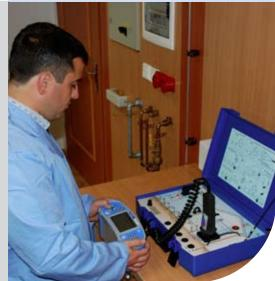
Demonstration board MI 2166 simulates common electrical installation usually met in individual house or apartment. Demonstration board is to be used preferably by sales personnel when demonstrating operation of electrical installation test equipment. Various test methods supported by different test instruments can be presented. MI 2166 is compatible with all Metrel's Installation Safety Testers.
