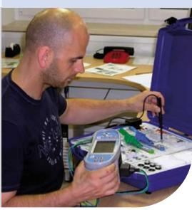
Demonstration board MI 3099 simulates typical electrical installation usually met in individual houses or apartments with important elements on switchboard and on circut site. Demonstration board is intended for use preferably by sales personnel when demonstrating operation of electrical installation test equipment, especially the new Metrel's electrically installations safety testers with built-in AUTOSEQUENCE procedure (MI 3101 EurotestAT and MI 3105 EurotestXA).
