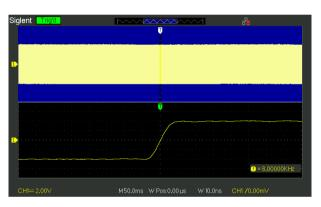
Zoom can extend a partial segment of the waveform, giving the user not only an overview of the whole signal but also a detailed view of the zoomed-in segment. The Zoom feature is a convenient way to locate a specific segment of a signal while zooming in to see the details.
