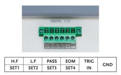
Another difference, while comparing with GDM-8251A, is that the Digital I/O of GDM-8351 provides two different modes which are general and self-definition. With the general mode, Digital I/O will output Hi Fail, Lo Fail, Pass and EOM (measurement results) based upon the results of the compare function and, furthermore, external trigger input is also provided. Under the self-definition mode, users can define output conditions for four pins (SET1~SET4) to execute the external control.
