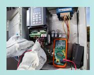
These professional DMMs are loaded with advanced features and functions. Low Impedance (LoZ) mode eliminates false readings caused by ghost voltages. Low Pass Filter (LPF)attenuates high frequencies to reduce noise for accurate readings. True RMS provides accurate readings when measuring distorted or noisy waveforms. Built-in Non-Contact AC Voltage Detector quickly checks for the presence of AC Voltage before testing.
