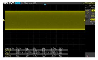
At any one timebase, the SDS1000X-E can measure using all 14M sample points. This ensures the accuracy of measurements while the math coprocessor decreases measurement time and increases ease-of-use.
