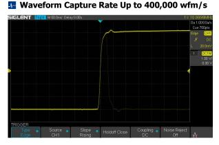
With a waveform capture rate of up to 400,000 wfm/s (sequence mode), the oscilloscope can easily capture the unusual or low-probability events.
