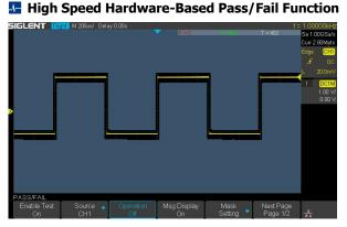
The SDS1000X-E utilizes a hardware-based Pass/Fail function, performing up to 40,000 Pass / Fail decisions each second. Easily generate userdefined test templates provide trace mask comparison making it suitable for long-term signal monitoring or automated production line testing.
