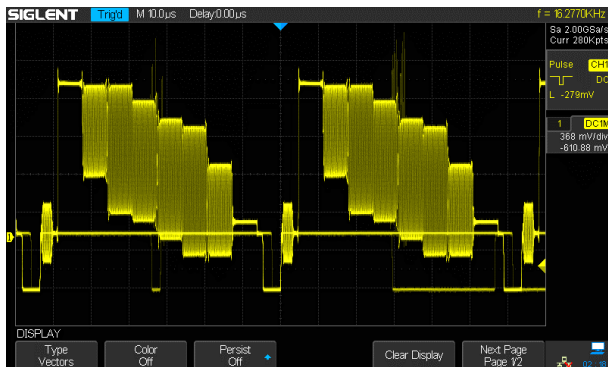
256-level intensity grading display on waveform
